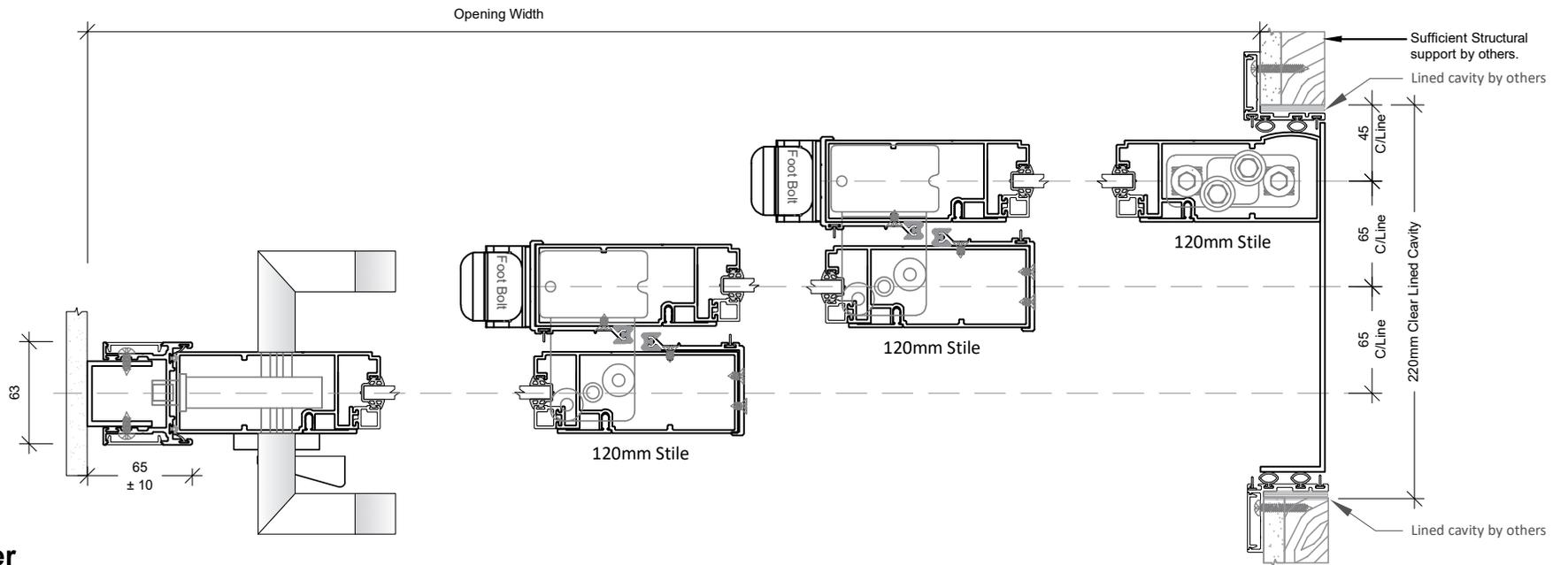
**Triple Cavity Slider**
