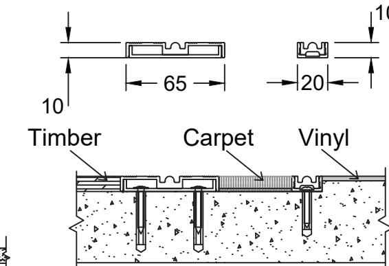
Floor track compatible with all finished floor types
