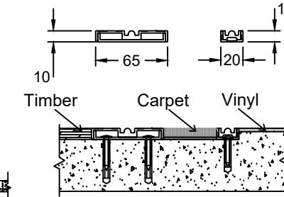
Floor track compatible with all finished floor types
